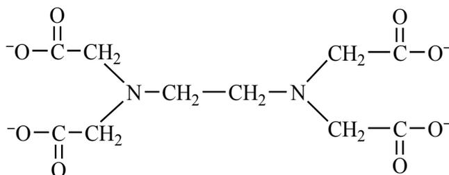
The EDTA ion is a hexadentate ligand and forms 1:1 complexes with metal ions. For example, nickel(II) ions react with EDTA ions to form a complex with the following octahedral structure:
