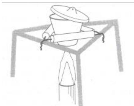
Heating is necessary to drive off any substances adhering to the surfaces of the crucible and lid. A blue flame is used to avoid sooty deposits. A significant error in the mass would result if this initial heating was not carried out or if a yellow flame was used.
