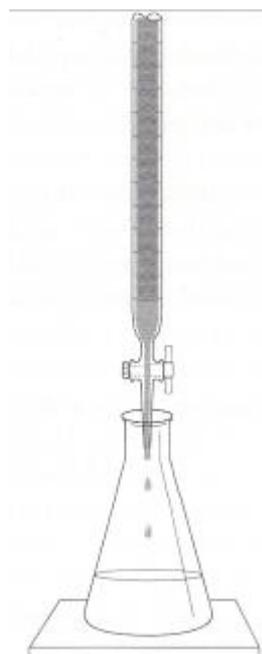
A second but more accurate titration is then performed. A portion of the analyte solution is pipetted into a clean conical flask along with a few drops
