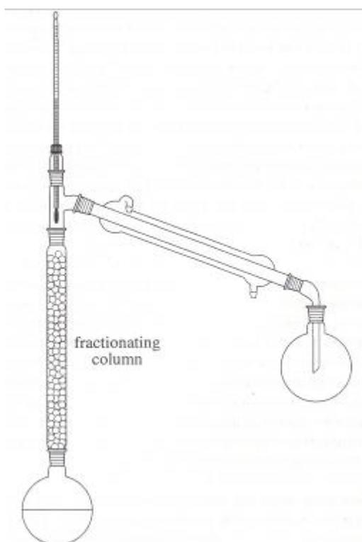
There are various types of fractionating column but the one illustrated above is packed with lots of tiny glass beads. Fractional distillation is a much more effective way of ridding a liquid product of impurities than simple distillation. The liquid mixture goes through a multi-step distillation as it rises up the fractionating column and a much ‘cleaner’ separation of the components takes place.
