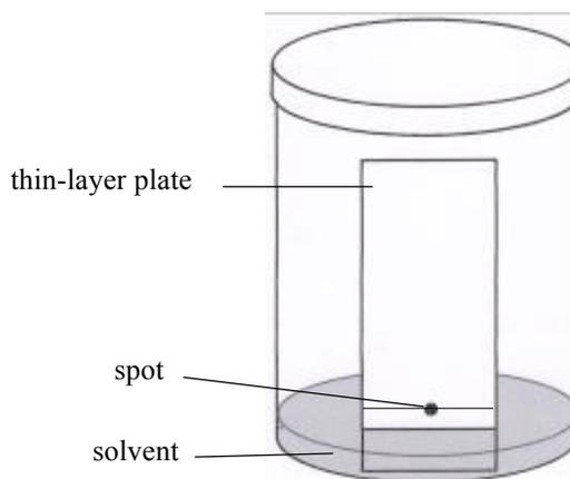
left to dry. This should be repeated two or three more times. It is important that the final spot should be about 1–2 mm in diameter. Once the spot is dry the plate is placed in a closed chamber with the lower edge (near the applied spot) immersed in a shallow layer of solvent, ie the mobile phase. It is important that the solvent level is below the line with the spot on it and that the chamber is closed completely. The latter ensures that the chamber is
