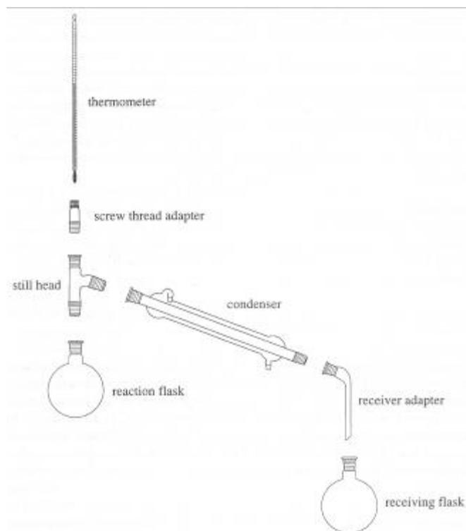
As in the preparation stage, the liquid mixture should occupy about half the volume of the round-bottomed distillation flask. The apparatus is then assembled as in the following diagram with the distillation flask sitting in a heating mantle and some fresh anti-bumping granules added to the mixture.
