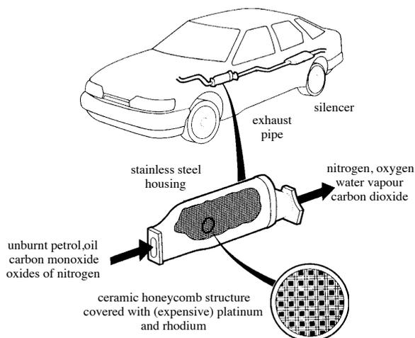
Converters are needed to change **harmful gases** into **less harmful gases**. Most have two sections:-
